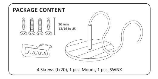
Mounting requires additional tools: 1 pencil + screwdriver. Attention: Table thickness should be over 20 mm (13/16 in US)
